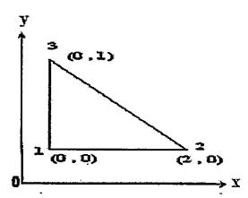
(b) Determine [B] and [D] matrices for axisymmetric element shown in figure. Assume E = 210 x  $10^3 \text{ N/mm}^2$ , Poisson's ratio  $\upsilon = 0.25$ . The coordinates are given in millimetres. [6M+6M]
