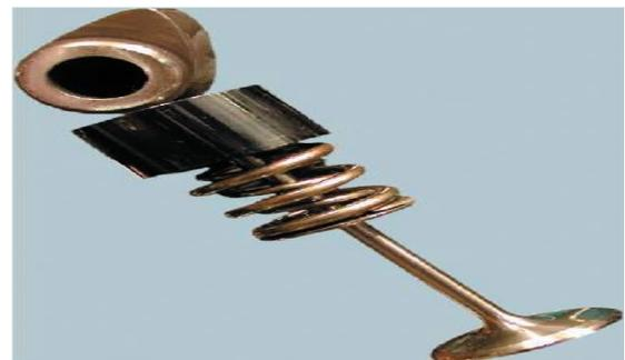
**Figure: The cam, cam tappet, valve, and valve springs**
