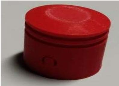
Figure 29:3D Printed Piston
