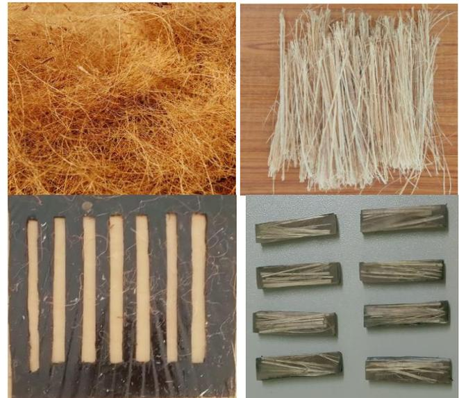
**Fig.1 (a) Corn Fiber, (b) Coconut Fiber, (c) Mould preparation, (d) Specimen for Thermal Conductivity Test, (e) Specimen for Impact test (f) Specimen for Tensile test**
