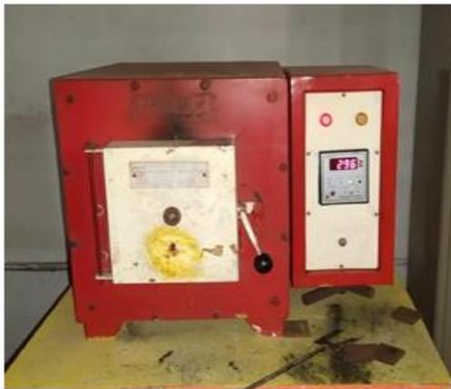
Fig 2: Muffle furnace
