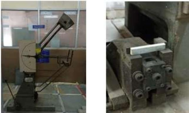
Fig.2.6 (a). Impact Test Machine, (b). Specimen fixed on testing machine
