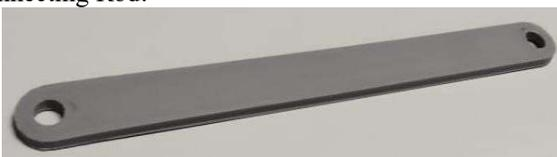
Figure 23:3D Printed Connecting Rod
