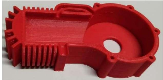
Figure 26:3D Printed Engine Case
