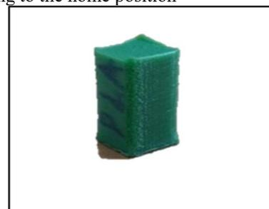
Fig.14 Printed Fatigue specimen
