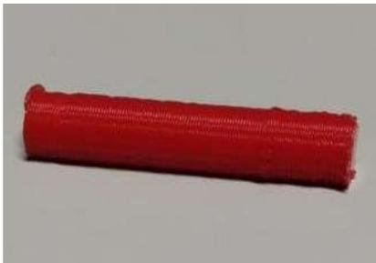
Figure 31:3D Printed Gudgen Pin
