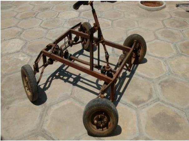
Figure28: Four Wheel Steering System
