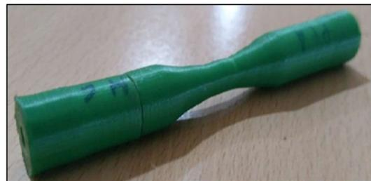
Fig. 13: Printed Fatigue specimen
