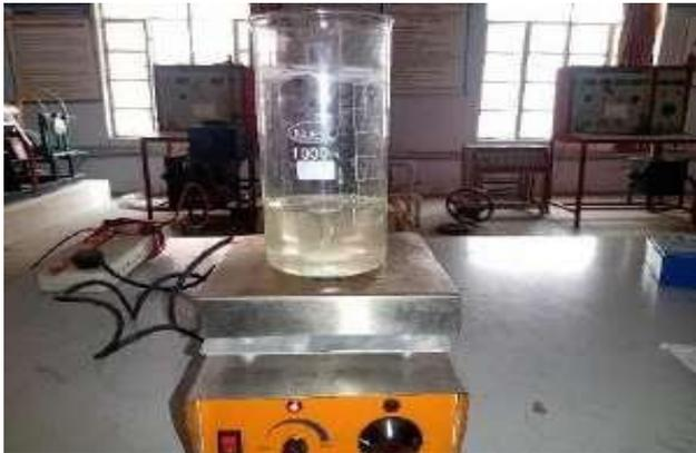
**Fig.2.1. Preparation of TiO<sub>2</sub> Nano lubricant were prepared (0.2g/L, 0.4g/L and 0.6g/L).**
