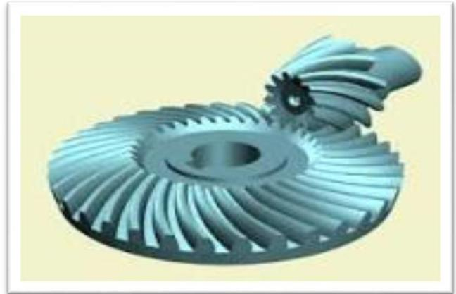
**Figure 3: SPIRAL BEVEL GEAR**
