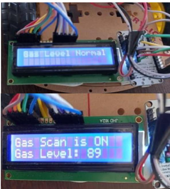
Fig.5.1 Gas Leakage level-Normal
