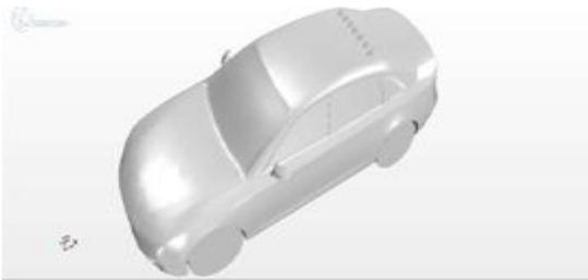
Fig 6: Geometry of Audi A4 with vortex generators
