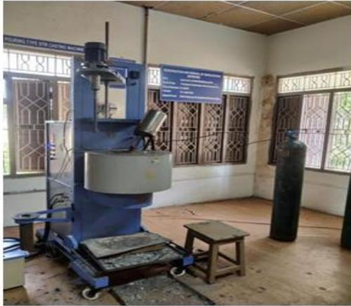
Fig 1: Stir Casting Equipment
