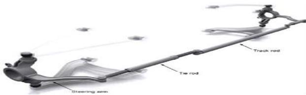
**Figure: 2 Conventional Front Wheel Steering System**
