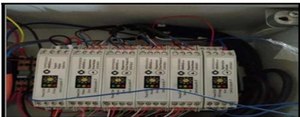
Fig 2: Programmable Logic Controller to Robot
