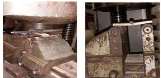
Fig.2.4. Specimen in bending test machine
