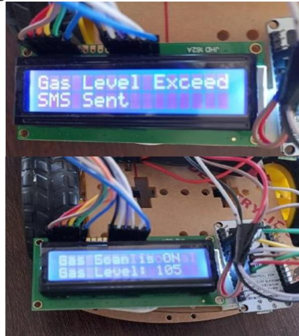
Fig.5.2 Gas Leakage level-Hig
