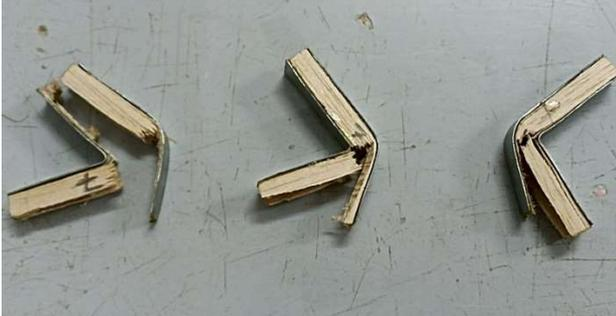
Fig.2.7. Specimens after impact test
