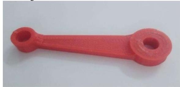
Figure 33:3D Printed Connecting Rod
