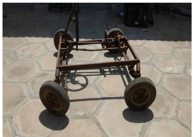
**Figure27: Two Wheel Steering System**
