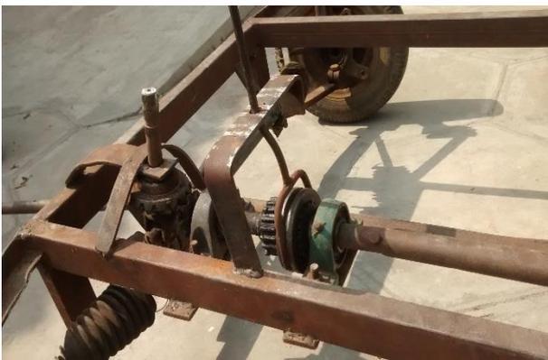
Figure29: Front Wheel Gearing System
