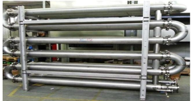
Figure 1.2 Shell and tube heat exchanger
