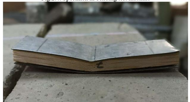
Fig.2.5. Specimen after bending test
