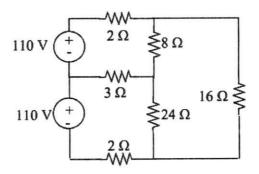
3. (a) Define incidence matrix. For the graph shown in figure, find the complete incidence matrix. 6M
