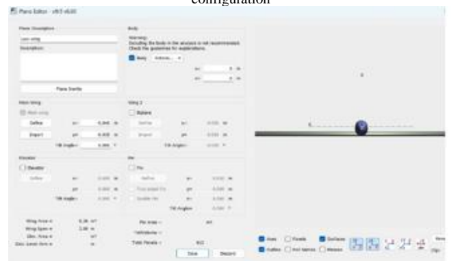
Figure-4.3: In the figure shows wing below Y- Axis means Low wing configuration
