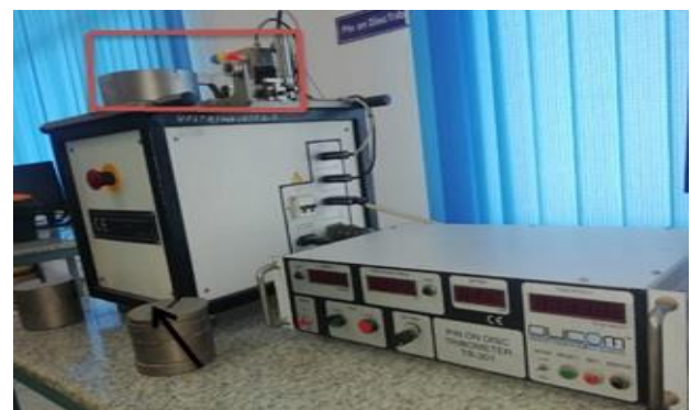
Figure 1.1: Wear Test (Pin on Disc Tribometer)
