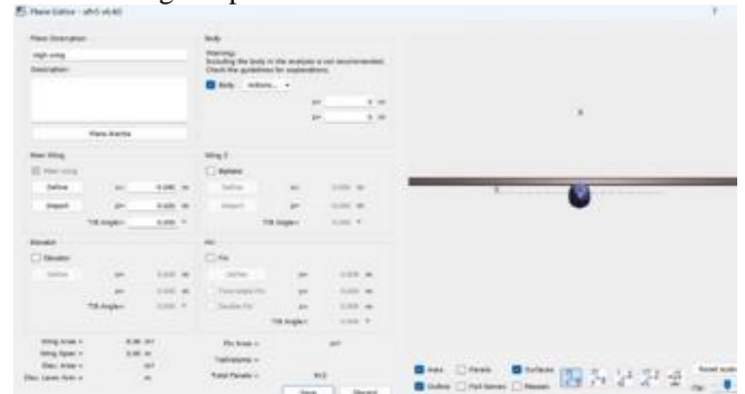
Figure-4.1: In the figure shows wing above Y- Axis means High wing configuration
