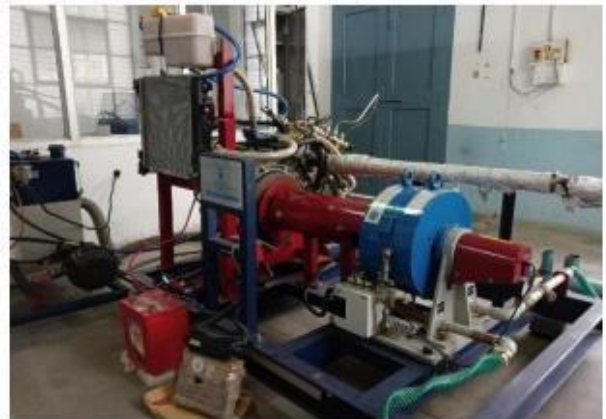
Figure 5: 4 stroke 1- cylinder diesel engine WITH EGR
