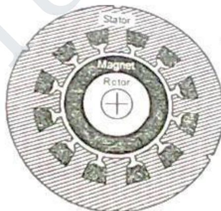
Fig 4.1 Arrangement of permanent magnet in the rotor
