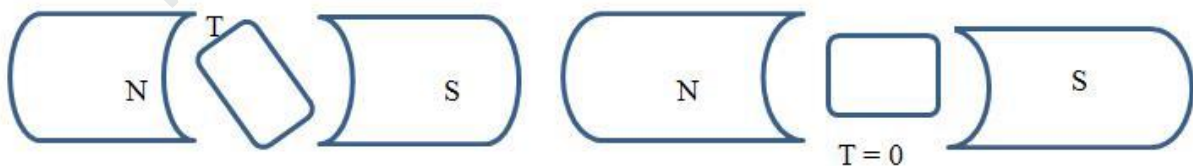
Fig1.10 Rotor Position due to Revolving Magnetic Field
