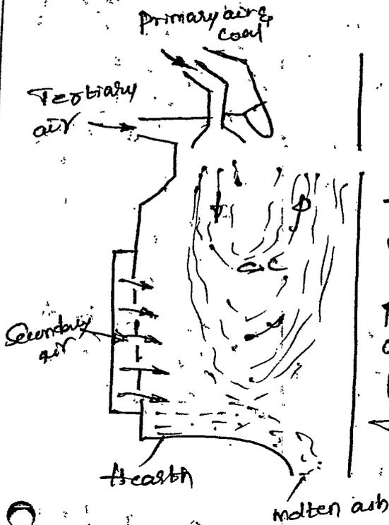
In this system tertiary air is supplied around the burner to form an envelope around primary air and fuel to provide better mixing. The burner discharges fuel and air mixture ~~is~~ vertically in thin flat streams with periodically no turbulence and produces a long flame. Heated secondary air is introduced at right angles to the flame which provides necessary mixing for better and rapid combustion.
