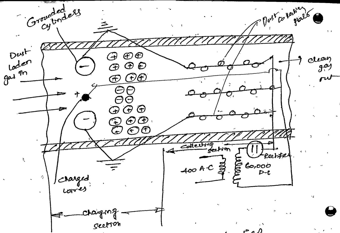
Layout of different components of ESP
