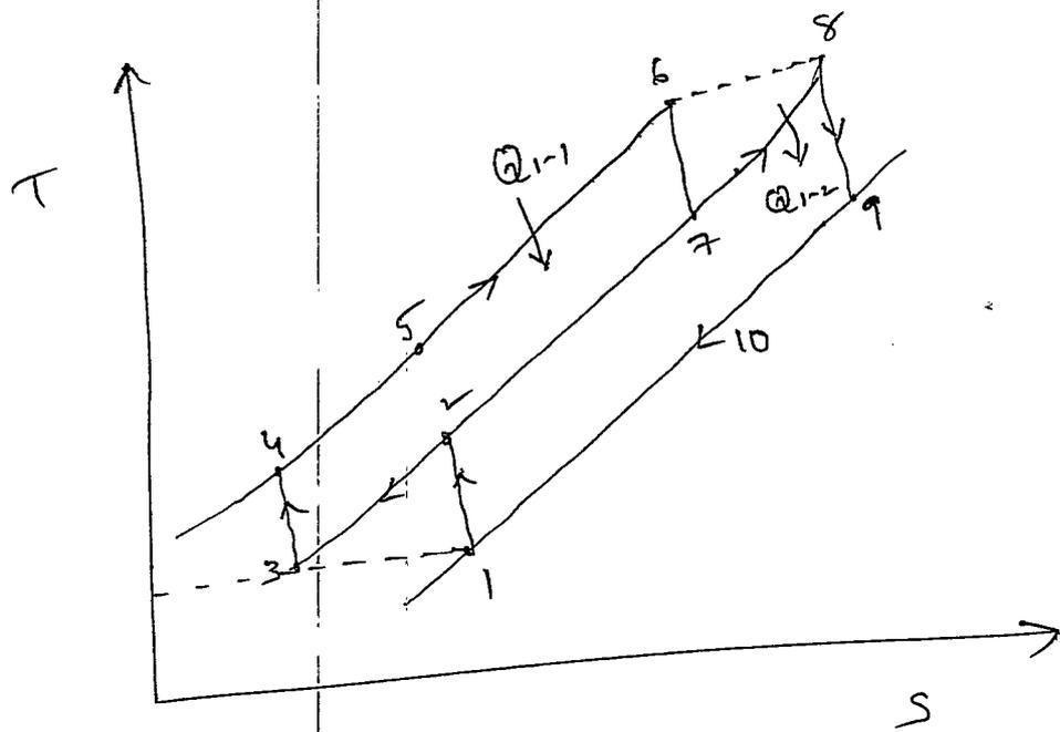
T-s diagram for Brayton cycle with Intercooling, Reheat & Regeneration.
