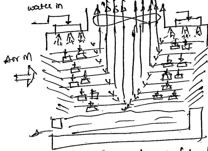
This tower provides horizontal air flow as water falls down the tower in the form of small droplets over falling. The fan centered at the top draws air through two cells that are joined to a suction chamber positioned beneath the fan. The drift eliminator turns air toward out let fan as air leaves the water spray. The outstanding feature of this tower is lower static pressure loss as there is less resistance to air flow.
