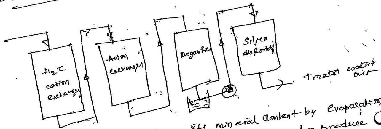
Water may be freed from its mineral content by evaporation or by series of cation & anion exchanger to produce distilled water. Then it is passed through degasifier & then the final exchanger absorb silica.
