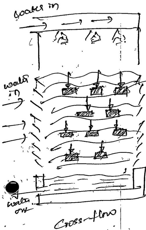
The construction of this tower is similar to spray filled tower except that water distributing troughs of jets are used which helps to break the water into small droplets. In this tower also the flow of air out air is cross wise to flow of water.
