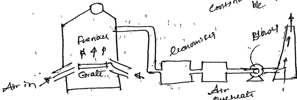
In this system the blower is located near the base of the chimney instead of near the grate. The air is sucked in the system by reducing the pressure in the system below atmospheric. Induced draught fan sucks the burned gases from the furnace & pressure inside the furnace is reduced below atmospheric & induces atmospheric air to flow through the furnace. Its action is similar to the chimney. The draught produced is independent of the temperature of the hot gases therefore the gases may be
