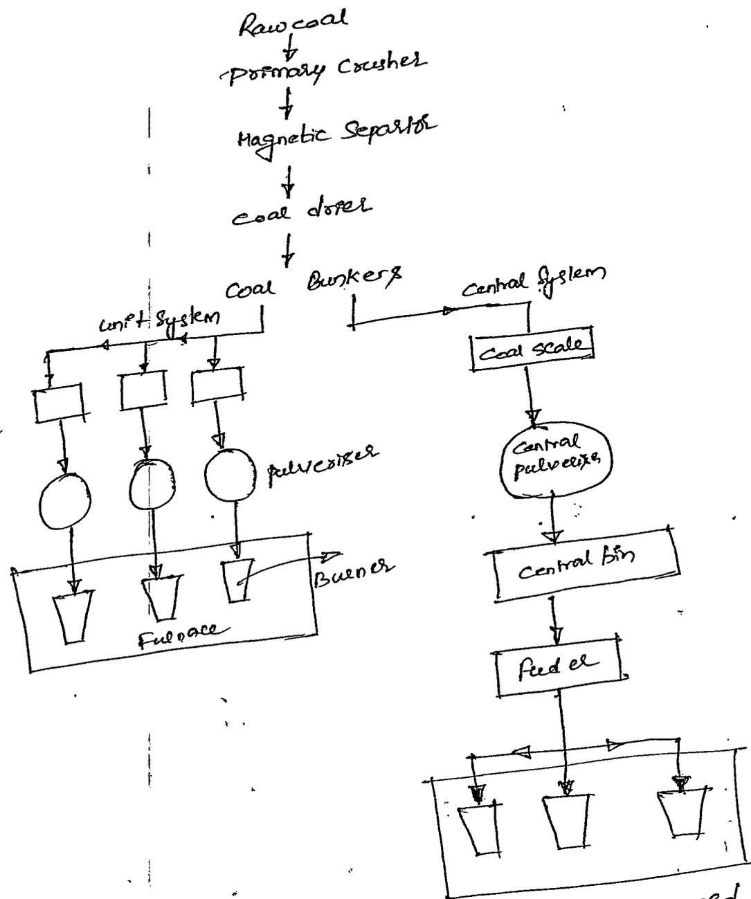
Pulverised coal handling plant showing all required for unit & central system.
