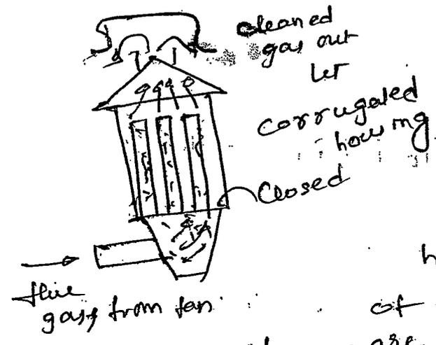
It is a closed air tight structure and fan is located to the inlet side of the bag house similar to open system. It is generally used for gases having DPT high DPT. The floor unit is closed and structure of the unit is insulated.
