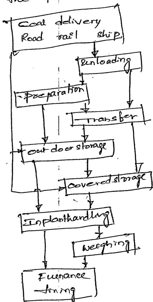
It is not necessary to follow flow chart for all the plants. Some intermediate steps may be eliminated depending on type of plant, capacity of plant & load factor.
