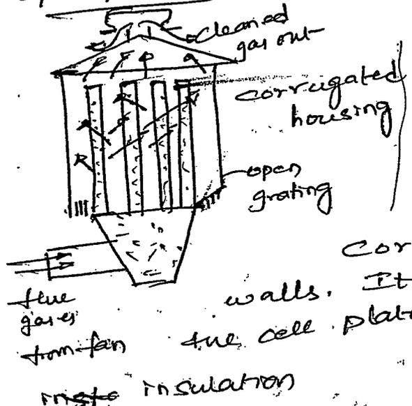
In open pressure bag house in which fan is located to the dust loaded side, can be operated with open sides as long as protection is provided from weather. This type is normally constructed with corrugated steel or asbestos cement walls. It may have open grating at the floor level. May not require hopper.
