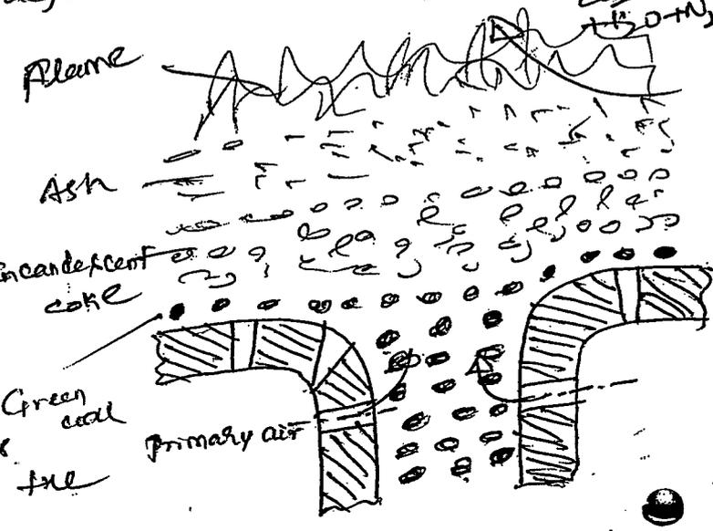
In this type of stokers the fuel & air move in the same direction.
