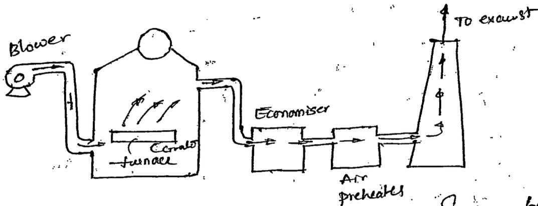
A stack or chimney is also used in this system but its function is to discharge gases high in the atmosphere to prevent the contamination. It is not so much significant for producing draught, therefore height of the chimney may not be very much.
