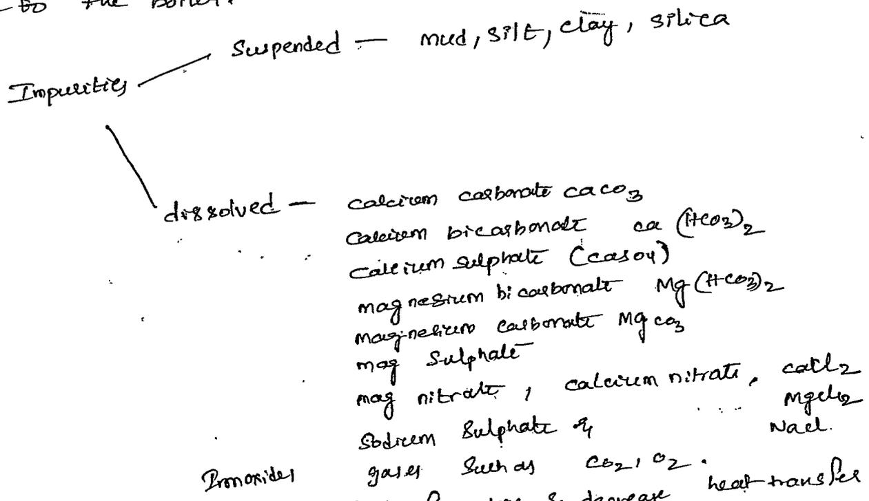
These impurities causes scales formation & decrease heat transfer & they restrict water flow through boiler tubes.
