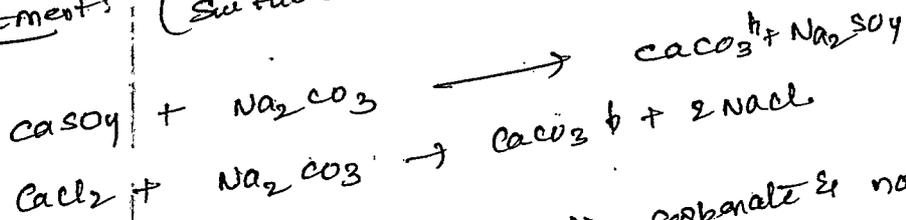
Lime soda treatment suitable if both carbonate & non carbonate hardness present
