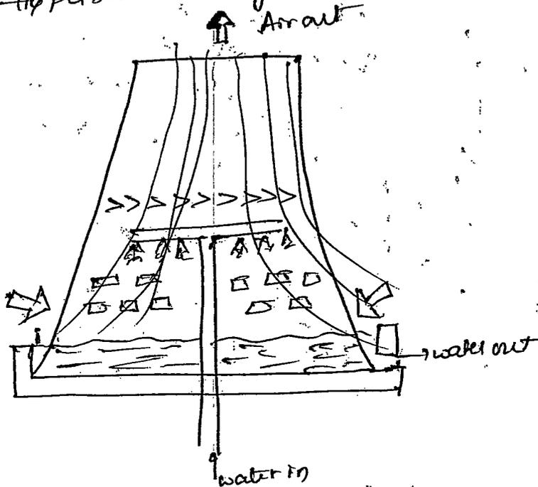
The cooling tower breaks the warm water into a spray or film of water & expose to flow of air. Some of heat in water is directly transferred to air stream & some of water evaporates providing sufficient cooling effect. Then the moist warm air goes to the atmosphere & cooled water is collected and returned to the power plant.
