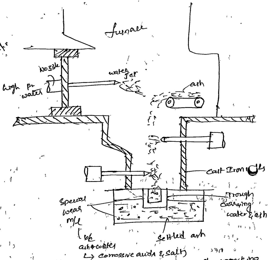
The important feature of this system is absence of working parts in contact with the ash.
