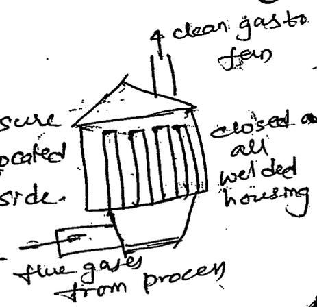
DPT from 15 to 85 °C. The floor, walls, and hopper of this unit are insulated. Blower maintenance is cheaper as it is located to clean side of gas.
