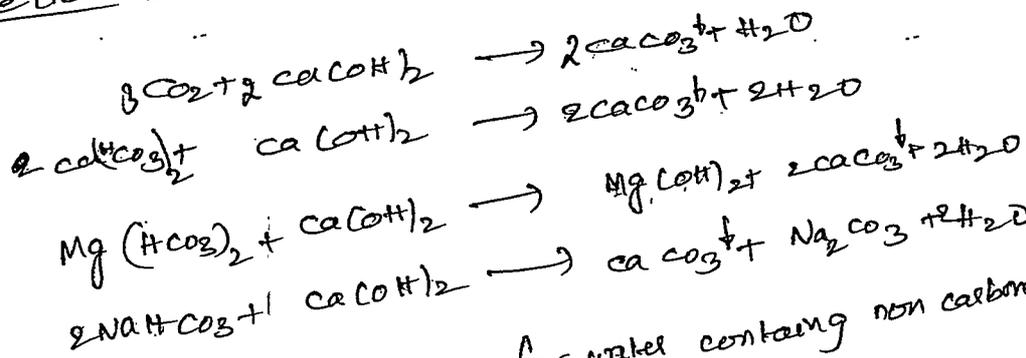
Soda treatment: (Suitable for water containing non carbonate impurities)
