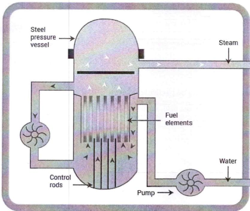
Pressurised heavy water reactor (PHWR)
