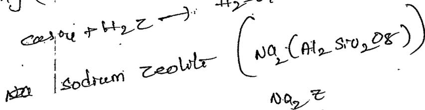
Zeolite can be regenerated through back washing with sodium chloride
