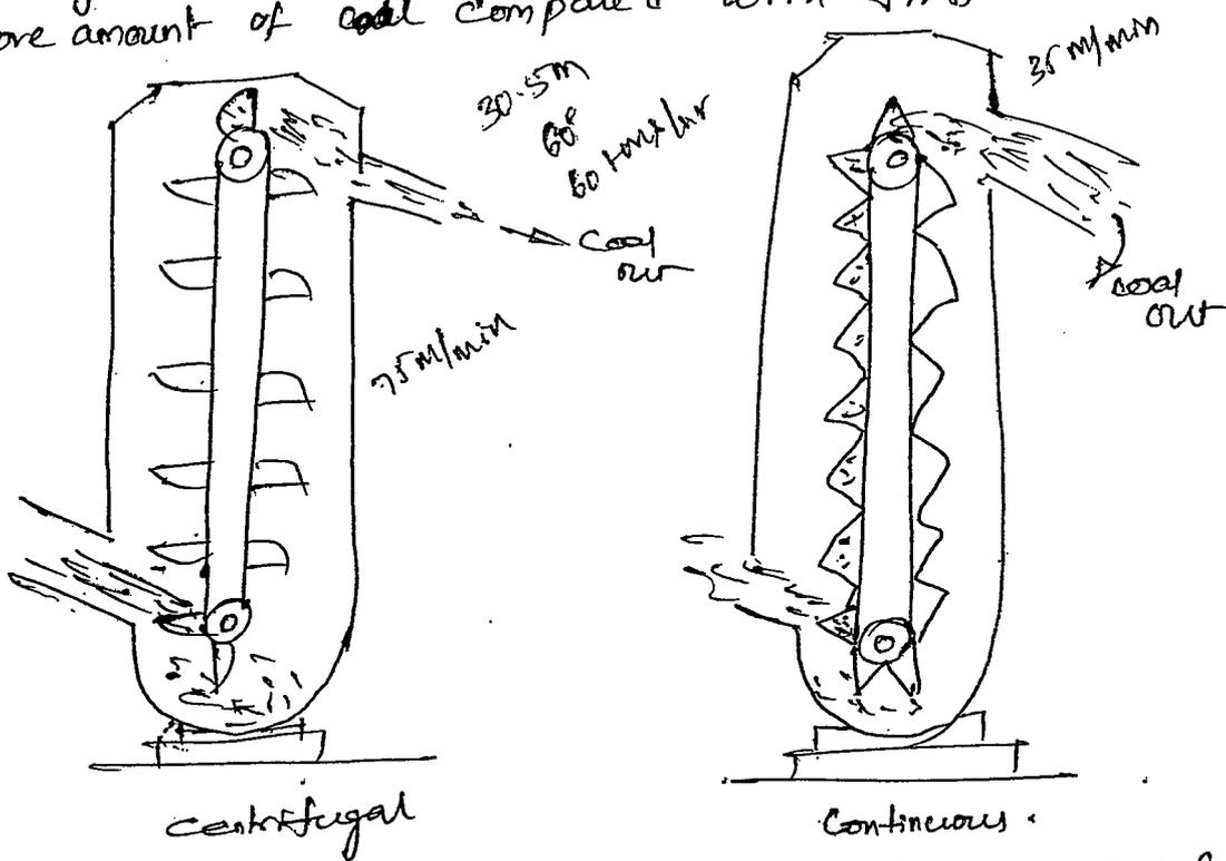
The max height of lift is limited to 30.5 m & max inclination to the horizontal is limited to 60°. The speed of chain required in first case is 75 m/min & continuous type is 35 m/min for about 60 tonnes capacity/hr.
