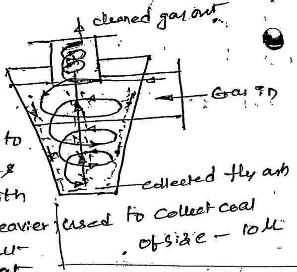
Some time multi cyclone dust collectors are used or multitubular type have been used extensively in process plants.
