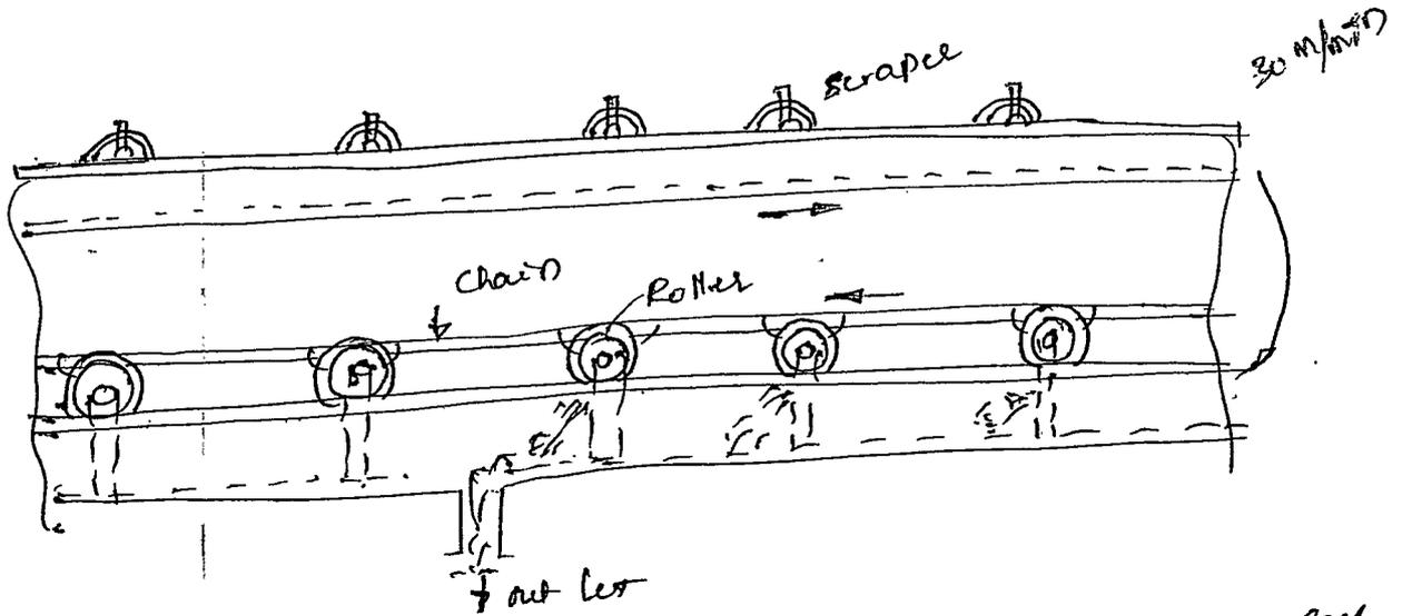
This conveyor is generally used for transfer of coal when filling a no. of storage bins situated under the conveyor is required. It consists of one or two strands of chain, to which steel scrapers are attached. The scrapers scrape coal through a trough & the coal is discharged at the bottom of the trough.
