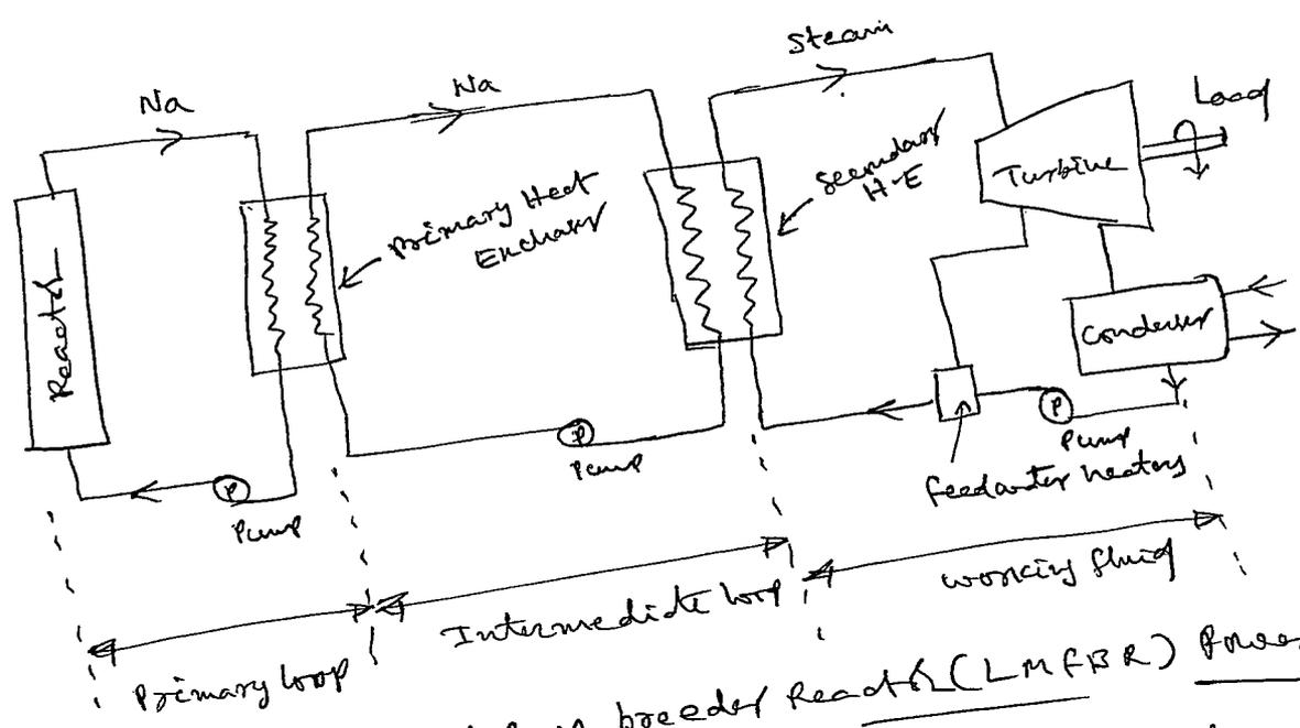
Liquid metal fast breeder reactor (LMFBR) power plant
