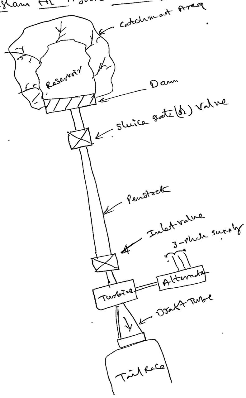
Flow sheet of hydro electric power plant
