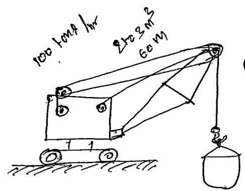
over a distance of 60m transfers nearly 100 tonnes per hour. The initial cost of this m/c is high but operation cost is less. Its use for transferring coal is justified only if volatile fuel is used only at up.
