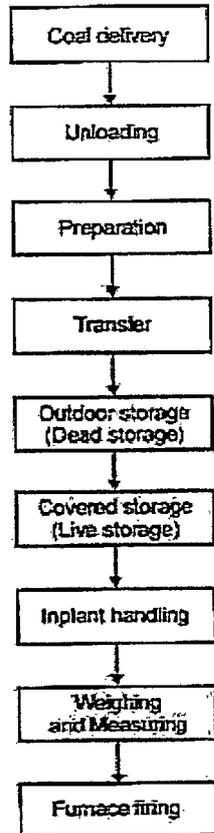
**Figure: Steps involved in fuel handling system**
