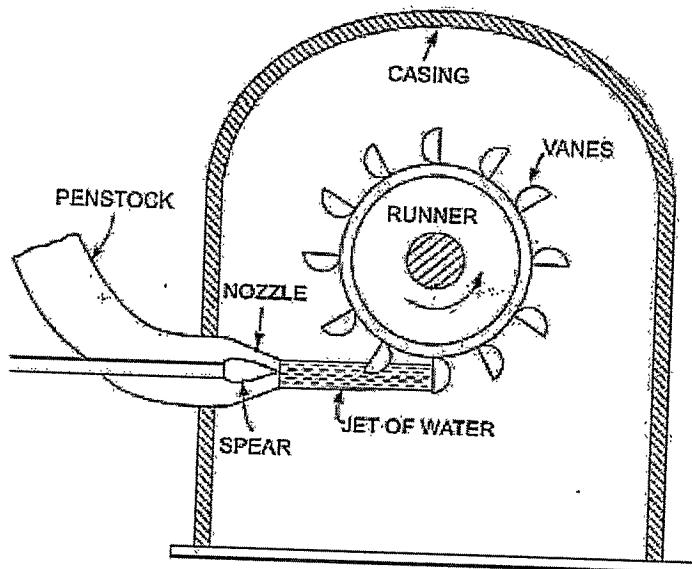
The main parts of the Pelton turbine are :
