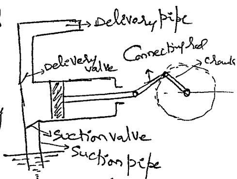
When piston moves towards the delivery pipe, pressure on the liquid increases and valve on the delivery pipe opens and liquid is pumped into the delivery pipe.
