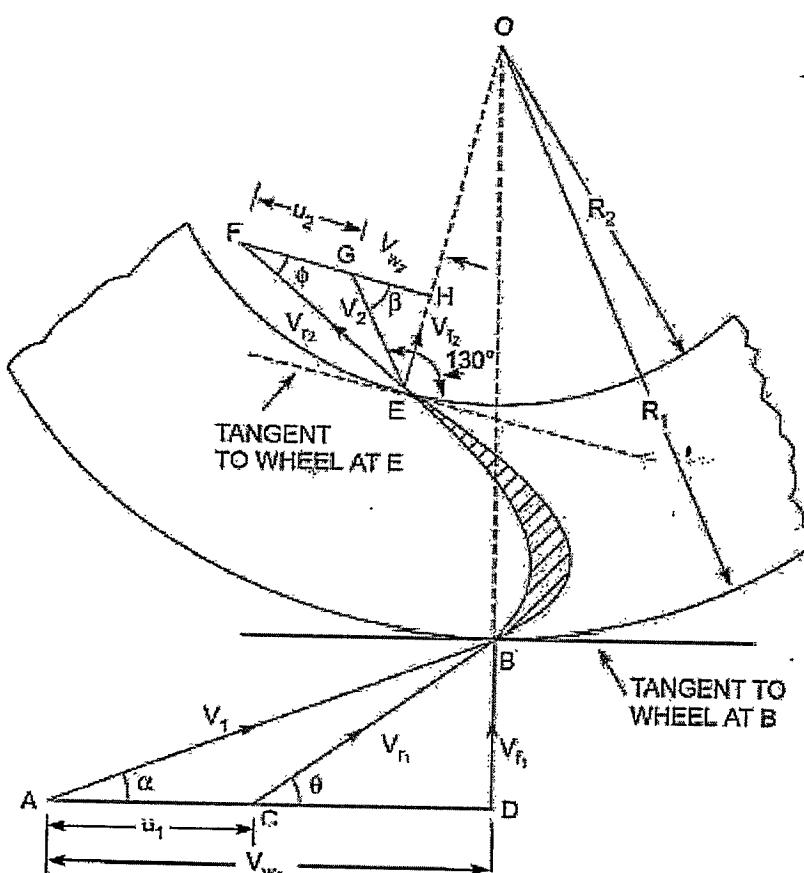
(i) Vane angles at inlet and outlet means the angle made by the relative velocities  $V_{r_1}$  and  $V_{r_2}$ , i.e., angle  $\theta$  and  $\phi$ .
