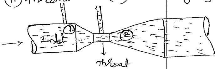
Consider a venturiometer fitted in a horizontal pipe through which a fluid is flowing. Let  $d_1, V_1, P_1$  and  $d_2, V_2, P_2$  are the diameters, velocities and pressures of the fluid at sections ① and ② respectively.
