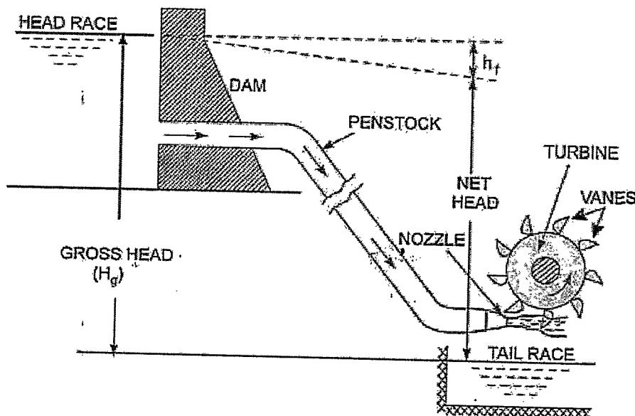
Fig. shows a general layout of a hydroelectric power plant which consists of :
