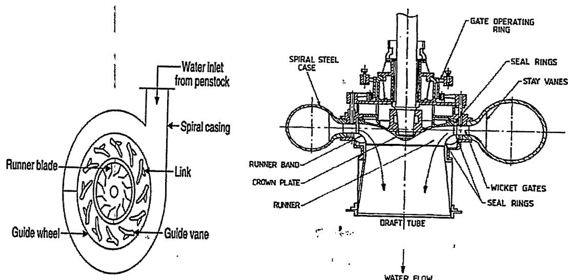
The velocity triangle at inlet and outlet of the Francis turbine are drawn in the same way as in case of inward flow reaction turbine. As in case of Francis turbine, the discharge is radial at outlet, the velocity of whirl at outlet (*i.e.*,  $V_{w_2}$ ) will be zero. Hence the work done by water on the runner per second will be
