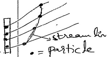
Streak lines are curved lines formed by a string of fluid particles which have passed through a certain point. These lines concentrate on fluid particles that have gone through a fixed station (or) point.
