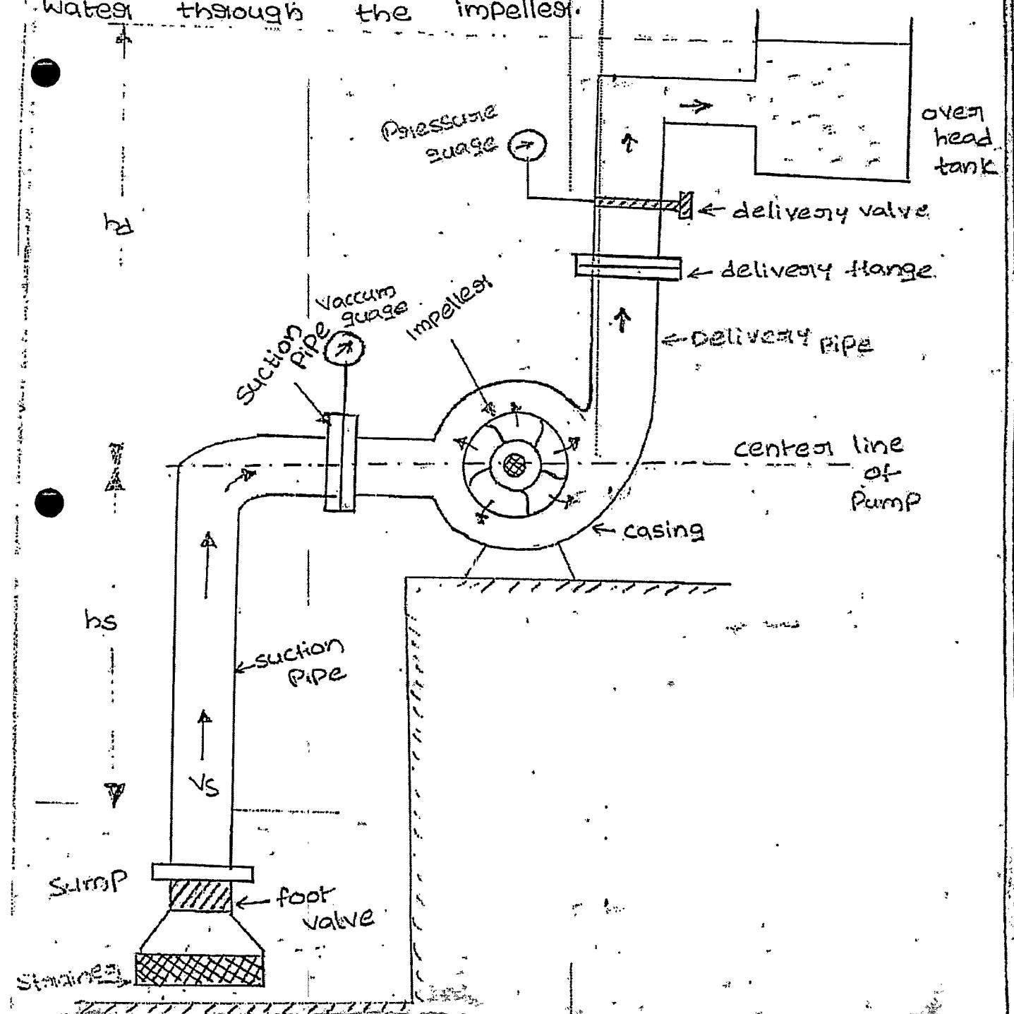
Casing: The casing is an air-tight chamber suspending the pump impeller. It contains suction and discharge arrangements, supporting for bearings and facilitates to house the motor assembly.
