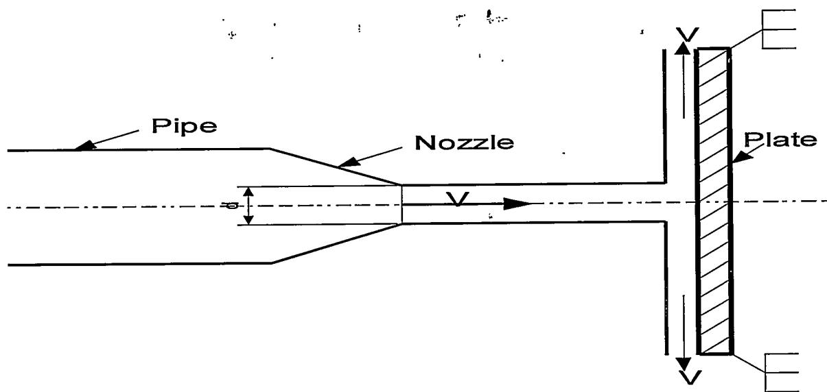
1. Force exerted by jet on vane in x-direction =  $F_x = \rho a v [v - 0] = \rho a v^2$
