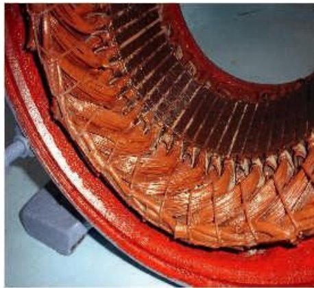
Figure 10: Coils in the stator
