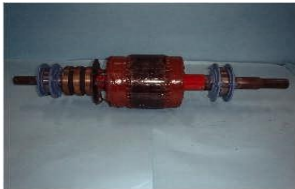
Figure 11: A wound rotor with slip rings
