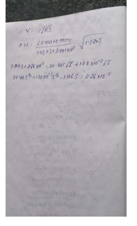
A Depign a channel for as us m3/s in non-alluvial Soil having maximum permaible velocity of o.9 mlp . the available bed Slope in 110 4000 Assume manningis 0:0025. Sept: Q: 45 m3/s V=0.9m/s 3 - 14000 n = 0.025 S'ide Blope = 0:501 Skp-2! Area, A: (b+md)d P: bt2d Titmv Q:AV V= 1 R23 5 12 V2 1/2 R235 1/2 09=0.025 R 3/3 / 4000) 1/2 0.9 = 40 R 2/3 × 0-015 0.9:0.632xR2/3 R=1-699 m A= 2/v = 45 = 50m<sup>v</sup> P= HR = 50 = 29.429
