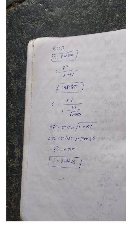
Design an isougation channel which carours on discharge 45 currecy & having Rugasty coefficient of 0.0223 & outral velocity ratio 1.03 having a bed slope of 11'n 5000. Given data, 0:450my 3:-1 11:0:025 m:1:05 Appume, D: 2.2m V: 0:055 x (2:2) 0:64 Nº 0.91 mlsec A= 0/v = 45 = 49.45 mv. A- BD+0/2 49.45 = B(2.2) + 12.00 B = 20:28 m P = 18+20 / 1464. P=18+D 15 25.19 P: 20:28 + 2(0.91) [1+ (0.545) P = 67.6 m
