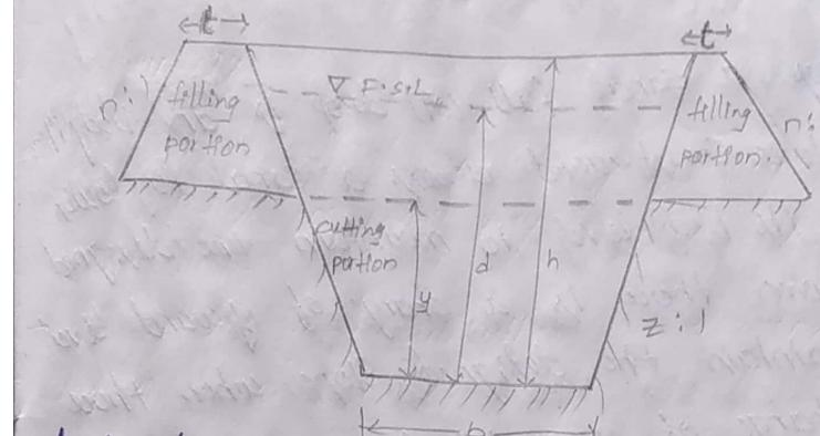
A channel section will be economical when the earth work involved at a particular section as ~~with~~<sup>an</sup> equal amount of cut and fill. For a channel section there will be one depth of cutting for which the cutting and filling will be equal this depth is known as balancing depth.
