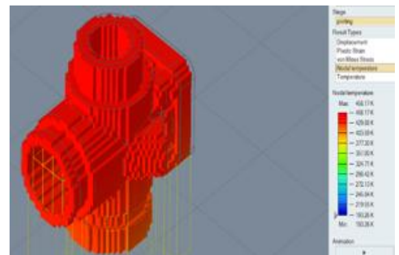
Figure: 9 Temperature distribution in second Orientation
