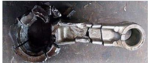
Fig 2: Connecting rod that initially failed through fatigue, the further damaged from impact with crankshaft
