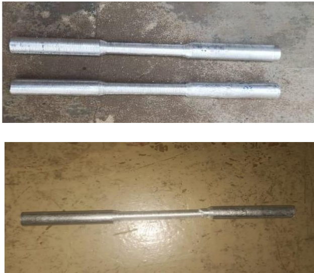
Figure 7: Samples of Tensile Before and After Testing
