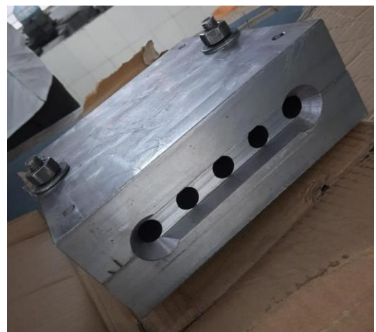
Figure 4: MS steel die block
