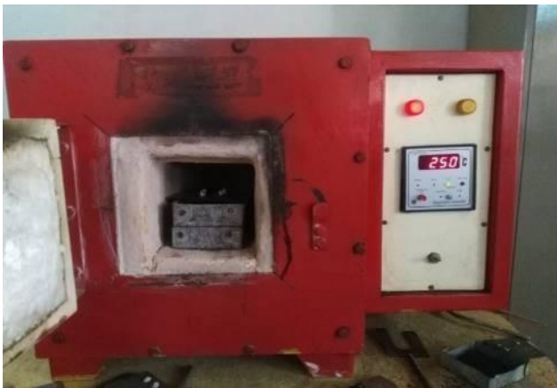
Figure 2: Pre Heating Furnace
