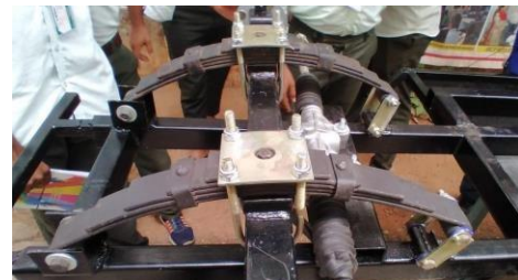
Fig 11 : Installation front wheel suspension
