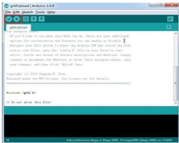
Figure 11. GRBL uploading into Arduino ide
