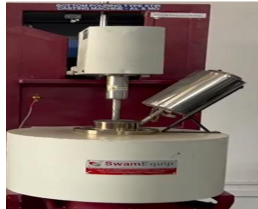
Figure 1: Photograph of stir casting setup
