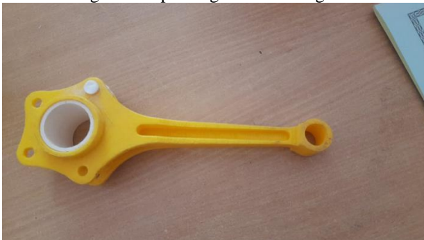
Figure 11 : final printing of connecting rod
