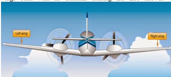
Fig.1.2.1 Left” and “right” wing of an aircraft to the perspective of a pilot sitting in the cockpit
