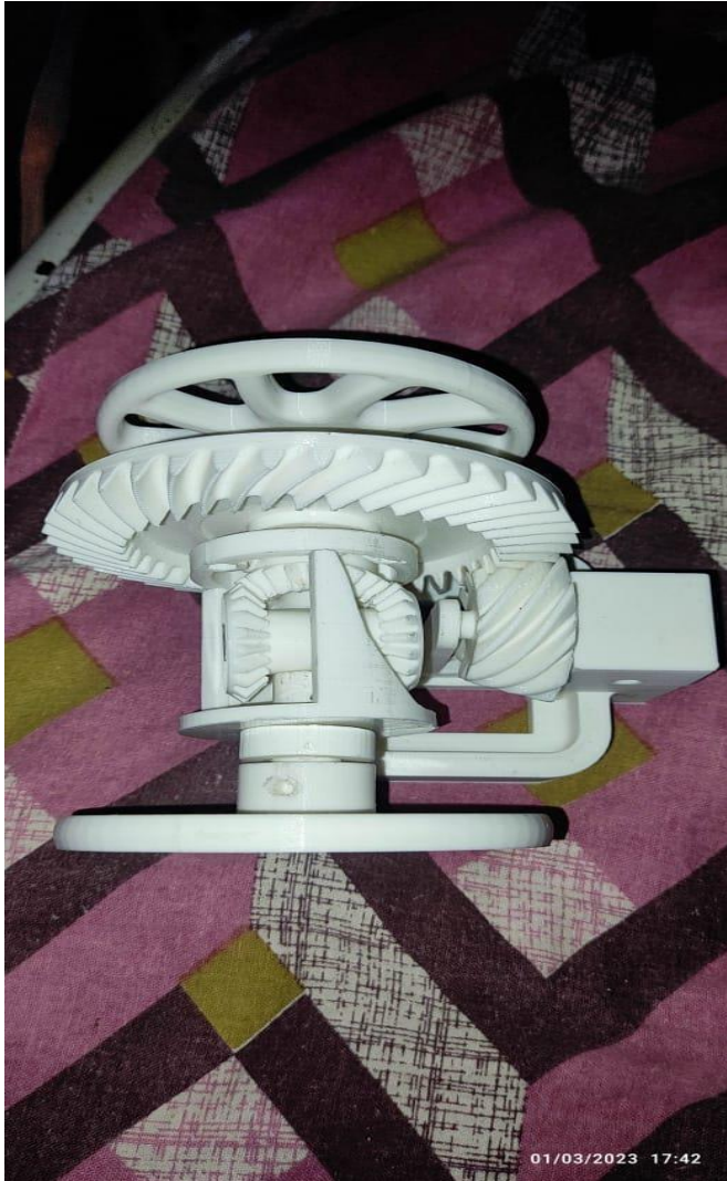
Fig.18: Final assembled Automotive Differential
