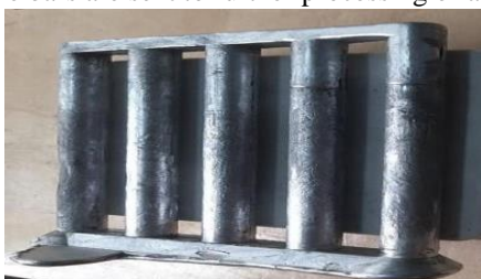
Fig:6. Produced A356-SiC Composite bars
