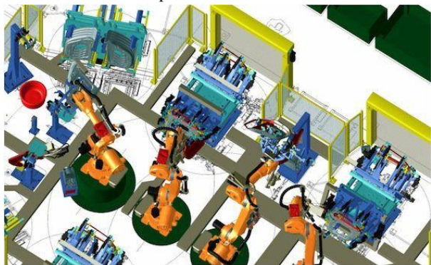
Robotic simulation using Robcad software for virtual manufacturing
