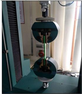
Fig. 4: Universal tensile testing machine
