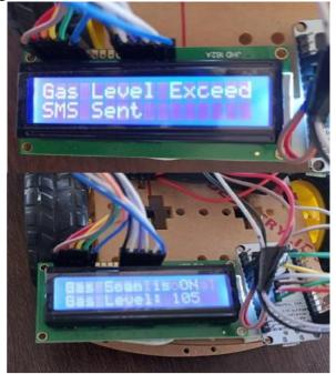
Fig.5.2 Gas Leakage level-Hig
