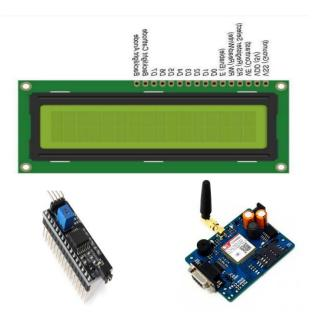
Figure 2.3 16\*2LCD Display, I2c display module & GSM800C module
