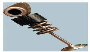
**Figure: The cam, cam tappet, valve, and valve springs** A cutout image cam-following mechanism in direct action is displayed, in shape bucket tappet working on valve with spring valve. This mechanism, like other cam followers devices, must during the planned work cycle in order to "trustfully" produce planned valve lift profile.
