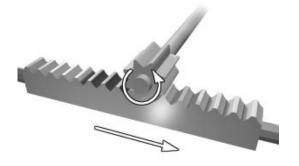
Figure22: Rack and pinion
