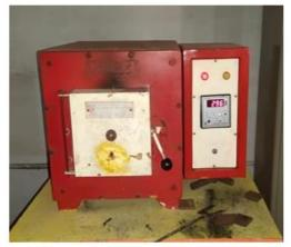
Fig 2: Muffle furnace
