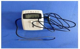
Monitoring the room air temperature: A digital thermometer is placed at the return air of the cooling unit inside the ripening chamber which records the return air temperature, which is the temperature of the air that picked the heat from the fruits and going to enter the cooling unit for lowering the temperature and to be blownagain on to the fruit crates. This instrument has been supplied by the supplier of the equipment, refrigeration unit of the ripening chamber.
