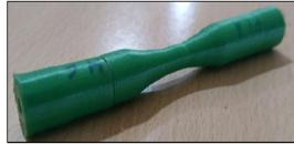
Fig. 13: Printed Fatigue specimen
