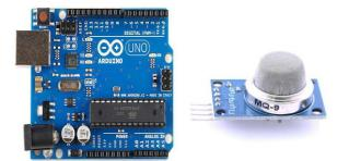
Figure 2.1.Arduino Uno Board & MQ-9 Gas Sensor
