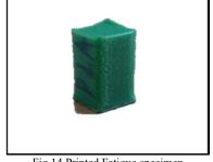
Fig.14 Printed Fatigue specimen
