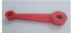
Figure 33:3D Printed Connecting Rod ASSEMBLING OF THE COMPONENTS AND PRINTING TIME Slider Crank
