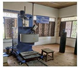
Fig 1: Stir Casting Equipment
