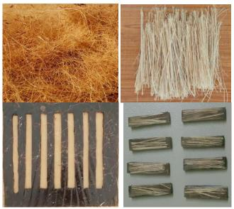
Fig.1 (a) Corn Fiber, (b) Coconut Fiber, (c) Mould preparation, (d) Specimen for Thermal Conductivity Test, (e) Specimen for Impact test (f) Specimen for Tensile test
