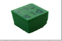
Fig. 12: Printed compression specimen
