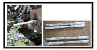
Fig: 14 Tensile Specimen preparation ; Fig: 15 Finished Tensile Specimen
