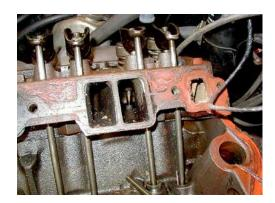
The cam actuates long rods that go up through the block and into the head to move the rockers. These long rods add mass to the system, which increases the load on the valve springs. This can limit the speed of pushrod engines; the overhead camshaft, which eliminates the pushrod from the system, is one of the engine technologies that made higher engine speeds possible.
