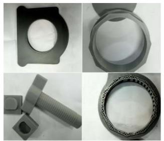
Total time taken for this print is 74 hours 45 minutes and the material consumed by the printer for this project is 360 grams. In cura software, arrangement of components were done in the effective way to reduce the time and material wastage.
