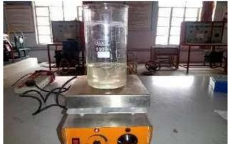
Fig.2.1.Preparation of TiO2 Nano lubricant were prepared (0.2g/L, 0.4g/L and 0.6g/L).
