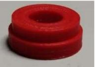
Figure 27:3D Printed bearing
