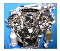
A double overhead cam engine has **two cams per head**. So inline engines have two cams, and V engines have four. Usually, double overhead cams are used on engines with four or more valves per cylinder -- a single camshaft simply cannot fit enough cam lobes to actuate all of those valves.
