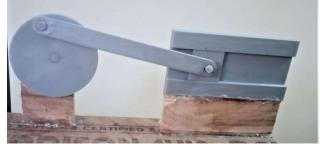
Figure 34: Assembled Component in single slider crank mechanism
