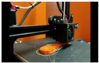
Fig. 4 Printing the 3D Object
