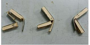
Fig.2.7. Specimens after impact test III. Results and Discussions 3.1 Experimental Observations from Tensile, Bending and Impact Tests: Table: 3.1 Tensile test results for G.I sheet
