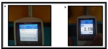
Fig.11 Surface Roughness tester with (a) Graph and (b) Value
