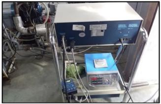
Figure 2. Photo graphical view of AVL 437 standard smoke meter
