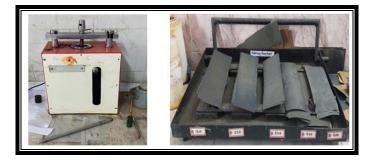
Fig: 7 Hot Mounting Press ; Fig: 8 Stand with different grit emery papers
