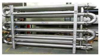
Figure 1.2 Shell and tube heat exchanger
