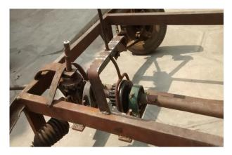
Figure29: Front Wheel Gearing System
