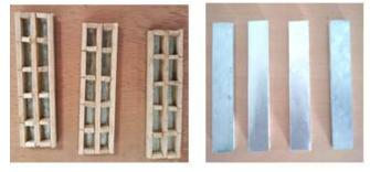
Fig.2.3. Bending test specimens
