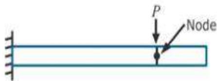
Concentrated load on a beam
