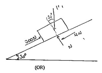
B) Determine force of p that will give the system of block shown fig 4.125 a velocity of 3m/s after moving a distsance of 4.5m from the position of rest. Coefficient of friction = 0.2  $[\cos x_1]$
