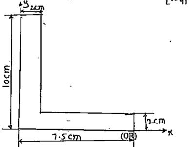
B) Calculate the moment of inertia of the shaded area with respect to a centroidal axis parallel to the x-axis.  $[Co_{ij}, \kappa_3]$
