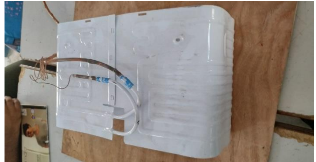
Fig 4.8 Evaporator for fabrication
