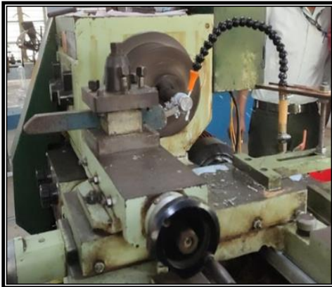
Fig 2. Automatic feed lathe machine with coolant
