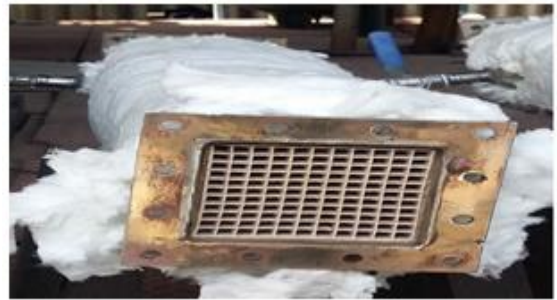
Figure 5: Pictorial view of 8mm Honeycomb & plate type SCR catalysts
