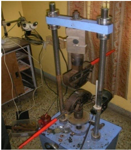
Tensile testing setup
