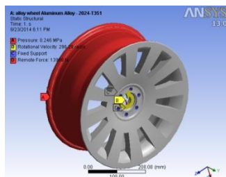
Fig.5 Pressure acting on the Wheel
