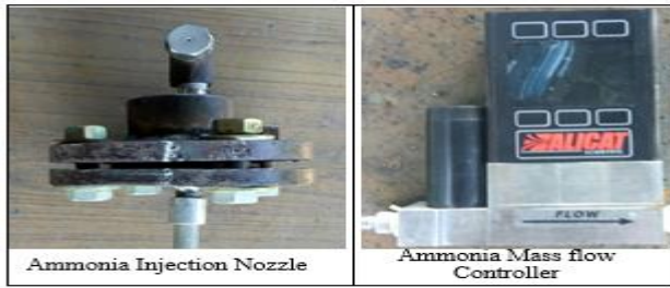
Figure 3: Anhydrous ammonia injection nozzle and mass flow controller
