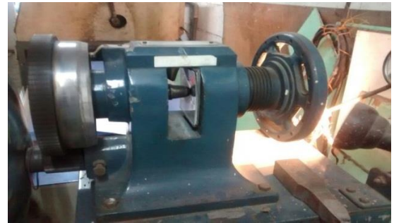
Ericission cupping test setup
