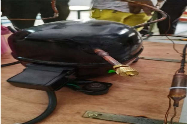
Figure- 4.5: Compressor used for fabrication
