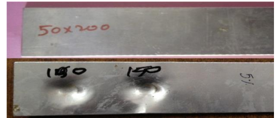
Impact resistance specimens before and after testing
