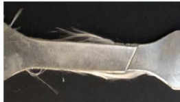
Tensile test specimens before and after testing.
