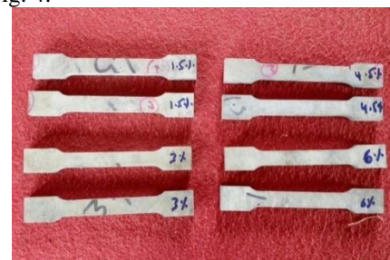
Fig. 5: Tensile test samples
