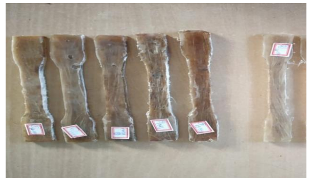
Fig.1 (a) Jute fiber, (b) Teak wood powder, (c) Chemical treatment, (d) Mould preparation, (e) Specimen for impact test (f) Specimen for tensile test
