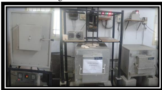
Fig. 2: Stir Casting Set-up used for fabrication of Composite Plates (Al 7075/WC)
