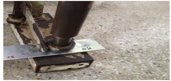
Impact Resistance test setup
