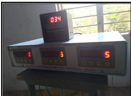
Figure 3. Tool dynamometer set up
