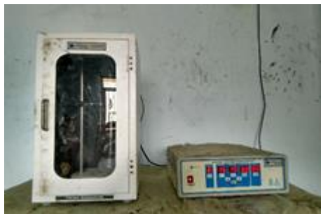
Figure 2: Ultrasonic probe sonicator
