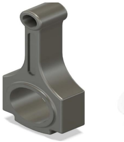
Fig 2 Connecting rod modelled in fusion 360.
