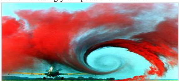
Fig1. A vortex is created by the passage of an aircraft wing, revealed by smoke. Vortices are one of the many phenomena associated with the study of aerodynamics
