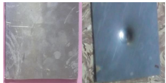
Ericission cupping test specimen before and after testing
