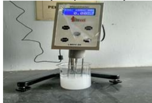
Figure 4: Viscosity measuring unit
