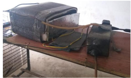
Fig-3. Condenser, absorber and evaporator unit.
