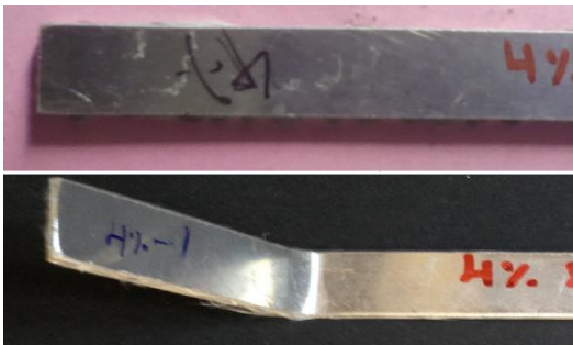
Flexural test specimens before and after testing
