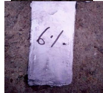
Fig. 3: Metal Matrix composite plates (Varying of WC content)
