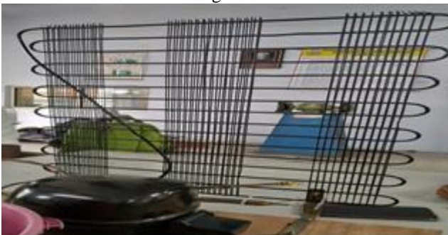
Figure 4.6: condenser used for fabrication
