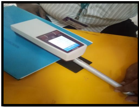
Fig 1. Surface Roughness Tester with work piece
